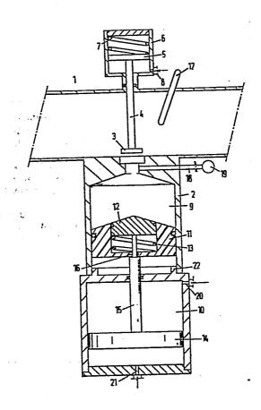
An apparatus for measuring the gas concentration of a gas-containing liquid.
