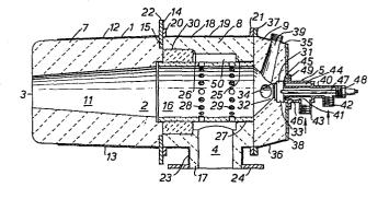
The present invention relates to a burner which, in one mode can serve as a burner per se and in an alternate mode as a flue for removing waste gas from a combustion space.
