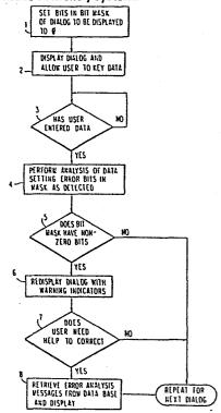
METHOD OF PROVIDING AN EXTENDED ERROR DIAGNOSIS TO ASSIST THE USER IN AN INTERACTIVE DATA ENTRY SYSTEM
