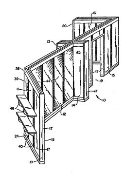
This invention relates generally to prefabricated walls, and more particularly to a prefabricated, free-standing wall having oppositely facing, exterior panels.
