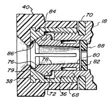
ELECTRODE GRIPPING ASSEMBLY FOR INCLUSION IN THE HEAD OF AN UNDERWATER CUTTING AND WELDING TORCH
