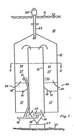
A device for increasing the oxygen concentration in a subsurface stratum of a thermally stratified body of water.
