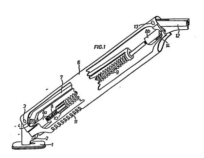
A supporting arm capable of being turned freely into different positions
