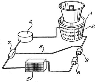
This invention relates to an ice-cream machine for family use with a whisking vessel which is removable from the ice-cream machine body, and in particular it relates to an ice-cream machine of the aforementioned type wherein new and higher usefulness is obtained in comparison with the ice-cream machines for family use known up to now, allowing in particular an easy removal of the whisking vessel from the ice-cream machine body.
