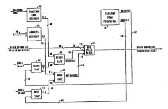
APPARATUS AND METHOD FOR SYNCHRONIZATION OF PERIPHERAL DEVICES VIA BUS CYCLE ALTERATION IN A MICROPROCESSOR IMPLEMENTED DATA PROCESSING SYSTEM
