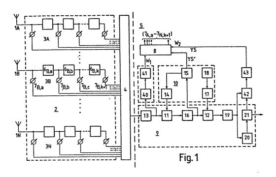
Communication receiving unit for the suppression of noise and interference signals.
