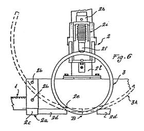
"AN APPARATUS FOR ABRADING MACHINING OF THE WELDING ZONE FOR THE RIMS OF BICYCLE AND MOTOR VEHICLE WHEELS".
