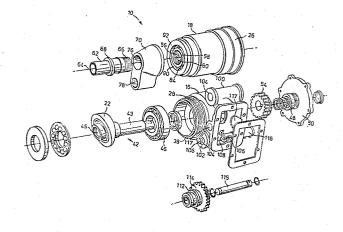
This invention relates to hydraulic wobble pumps. In particular, this invention relates to improvements in wobble pumps which permit even distribution of the incoming hydraulic fluid to the various cylinders of the pump and facilitate the removal of the power transmission gearing.
