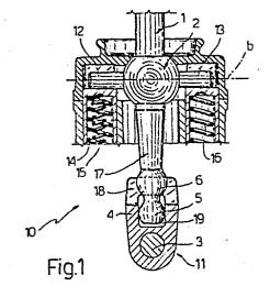
"Transmission gear shift and control device, particularly for industrial vehicles"
