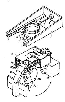
An apparatus for X-ray photography of the area of the dentition and the jaws
