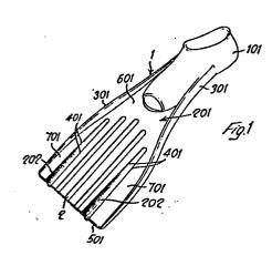
Swim fin provided with a self-shaping, fluid flow conveying and controlling canal-like member.
