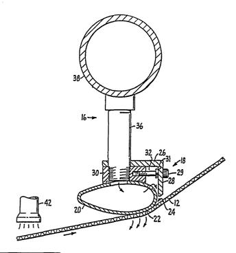
This invention relates to a method and an apparatus for cleaning and conditioning fabrics, e.g. felts and wires on a papermaking machine.
