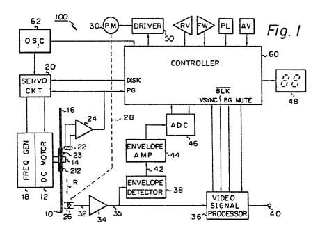
TRACKING APPARATUS FOR ROTARY MAGNETIC RECORDING MEDIUM
