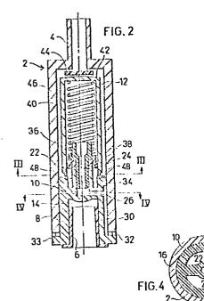
The present invention relates to a quick-action on/off valve. More particularly, the invention relates to a valve which effects a quick-action opening of the line when the line pressure reaches a predetermined minimum, and effects a quick-action closing of the line when the line pressure drops below a predetermined minimum.
