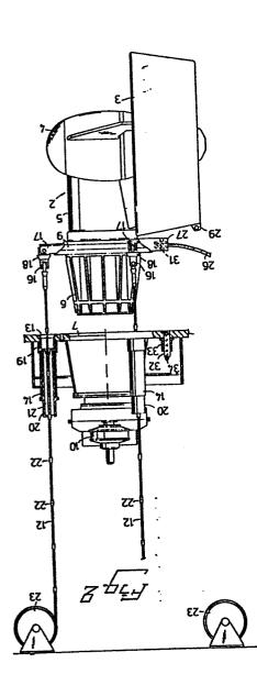
An arrangement for fitting a propeller assembly to an opening in a bottom structure of a watercraft and for dismantling the assembly therefrom.
