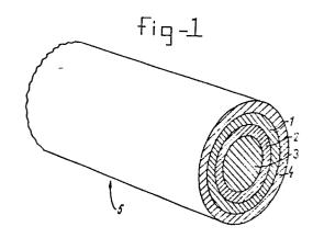
A method for the manufacture of a superconductor in the form of a single-filament or multi-filament wire or tape, and superconductor manufactured in this way.
