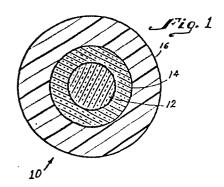
This invention relates to optical fibers and more particularly to optical fibers coated with a single ultraviolet-cured resin and which is particularly useful in cables where the fibers are loosely contained.
