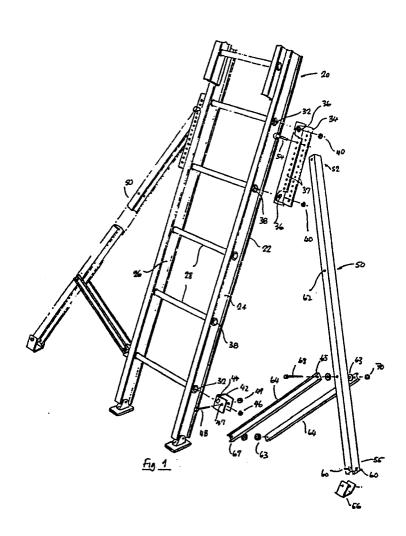
The present invention relates to a ladder stabilising device for extension ladders having hollow rungs. More particularly, the invention relates to an adjustable ladder stabilising device which can be secured to one or to both sides of the ladder without interrupting the structural integrity of the ladder.
