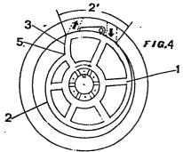
"A device with a rotating piston provided with an arc portion and a spiral profile for supercharger and fluid motors"
