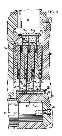
This invention is in the field of multiple disk refiners employing sets of stationary spaced stator disks and refiner rotor disks between which are provided
