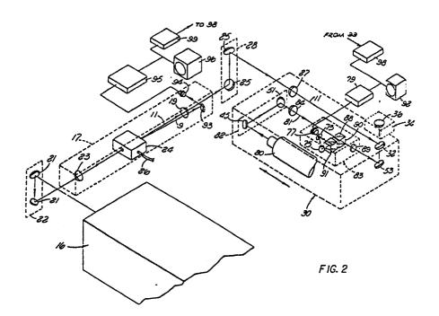
This invention relates generally to improvements in video recorder-playback machines, and more specifically to an improved arrangement of optical components in a video recorder-playback machine of the type including optical laser beams for recording and playback of video information from a video information disc.
