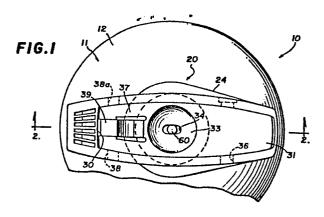
The present invention relates to valve mechanisms for controlling the discharge of material under pressure from a container. In particular, the invention relates to discharge valves for fire extinguishers.
