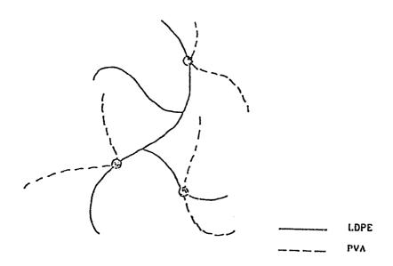
Fig. 2. Ethylene/vinylalcohol segment mixed polymer.
