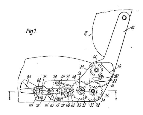
The present invention relates to automotive seat recliners and, more particularly, to a manual clutch release seat recliner having a gearing mechanism to permit the controlled reclining of an automotive seat back.
