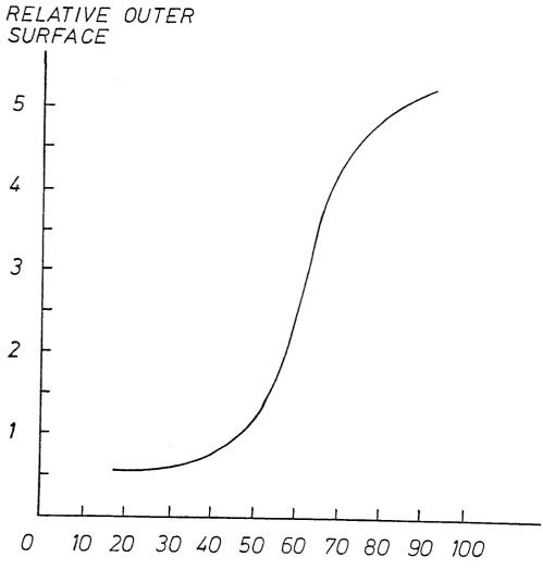
% OF TOTAL FIBRE LENGTH DEVIATING BY AT MOST 20° FROM MAIN ORIENTATION PLANE
