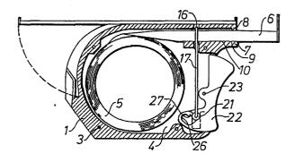
The present invention relates to a locking device for a scale in a tool with combined length marking and measuring functions, where the scale is printed on an arched tape which may be rolled up and is made of steel or other greatly durable material. The tape is disposed in the form of a roll in a housing associated with the tool, from which the tape is withdrawable. Similar combination tools, so called mark meters, are known from the Swedish patents Nos. 152.749 and 175.653.
