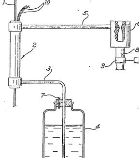
This invention relates to gas chromatographic analysis equipments and concerns a method and a device to adjust the cooling temperature of a trap for samples to be analysed.
