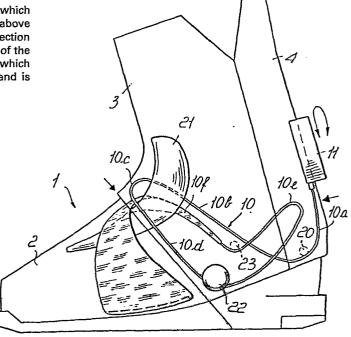
"SKI BOOT WITH A MECHANISM FOR SECURING A FOOT INSTEP AND HEEL"
