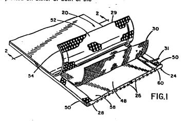
plates pierce the web material between the conductors in the flat cable as the body and cover close so slitting of the cable between conductors is not required.
