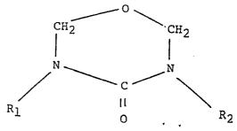
where  $R_1$  and  $R_2$  are H. -CH<sub>2</sub>OH or alkyloxymethyl. and subsequently heat-curing the resin in the fabric. is carried out with a polyol having 2 to 4 carbon atoms, such as diethylene glycol, in the solution to inhibit the build-up of solids on heated elements which the impregnated fabric contacts during processing.
