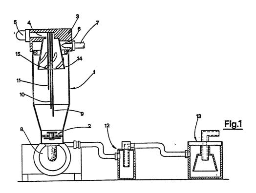
A spittle separation and disposal device incorporating a drainage pump, in particular for suction equipment used in dentistry.
