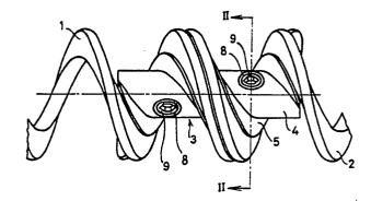
CONNECTION MEANS FOR SUCCESSIVE SECTIONS OF A HELICAL SPRING LIKE CONVEYING ELEMENT.
