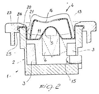
"An electrical switch having a sealing element, particularly designed for window winders"
