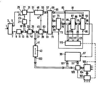
Teletext signal processing circuit for a teletext receiver.
