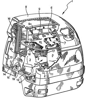
Lorry cab having a driving position and a rest position with bunks.
