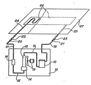
The present invention concerns a cooling unit for coffins, of the type using a refrigerating circuit consisting of a compressor, a condenser, one or more expansion or similar valves and an evaporator, which is in a situation of heat exchange with the interior of the coffin.
