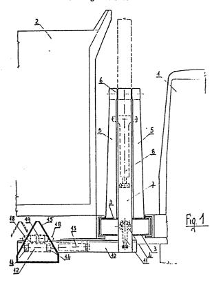
Device for lifting, tilting and discharging of garbage containers into the garbage truck, fitted with removable slide, one or more lever arms and hook-up by means of an oscillating and transverse mobile triangular head
