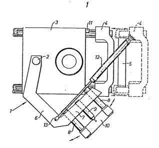
The invention relates to a core setter for use in placing one or more cores in the mould impression in the rearmost of a number of mould parts or in the mould impression on the front of the subsequent mould part during conveyance from the moulding chamber, such mould part having been made in a vertical moulding system and during conveyance towards a pouring line.
