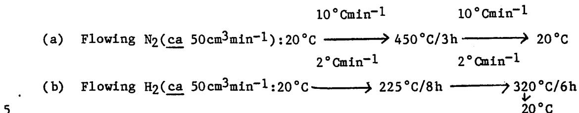
The heat-treated catalyst was exposed to air and stored in air in screw-top jars.
