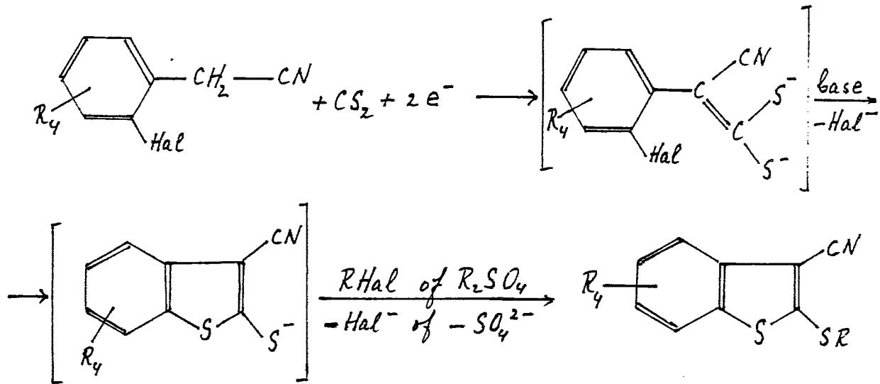
25 The first reaction step can be carried out by reacting the starting substance, in which Hal is a halogen atom, with CS<sub>2</sub> under the influence of a suitable base, for example, sodium hydride, preferably in a polar organic solvent, for example, DMF, at a temperature between 0°C and the boiling point of the solvent. The subsequent reactions can be carried out in the same manner as corresponding, previously described reactions.
