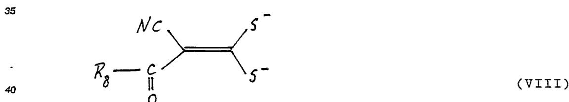
50 successively with a compound of the general formula R<sub>1</sub>-CH<sub>2</sub>-Hal and with a compound of the general formula RHal, wherein Hal is a halogen atom. The reactions are preferably carried out in a polar organic solvent, for example, DMF, at a temperature between 0°C and the boiling-point of the solvent.
