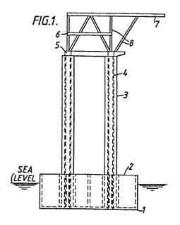
This invention relates to offshore structures and, more particularly, to structures utilized as oil or gas production platforms.
