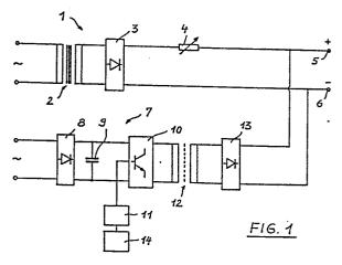
ARRANGEMENT FOR THE GENERATION OF A WELDING CURRENT HAVING A D.C. PORTION AND SUPERIMPOSED CURRENT PULSES
