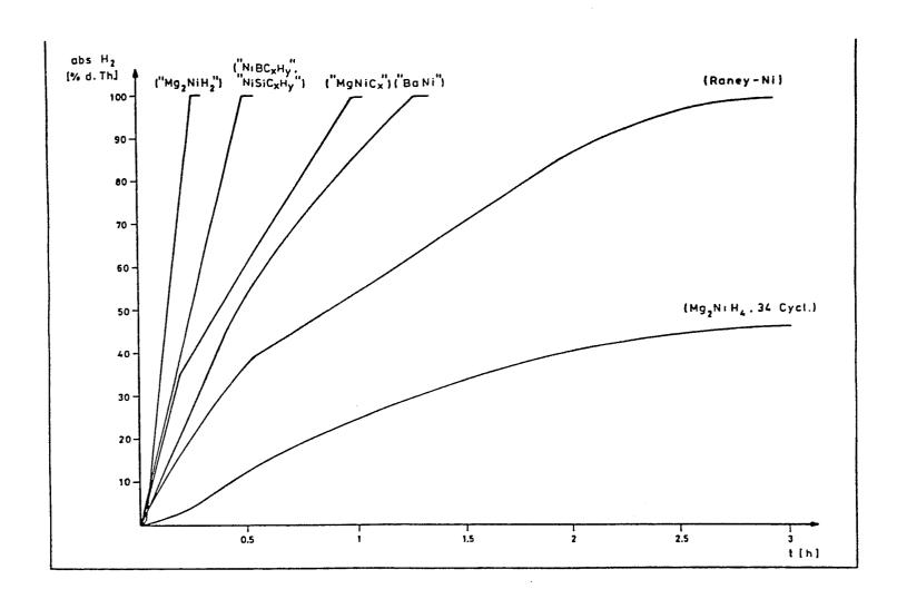
Figure 1: Catalytic hydrogenation of a mixture of cylohexene and heptene-1 using some metal nickel compounds as catalysts (room temperature, normal pressure, ratio of olefinic group:Ni = 40:1).
