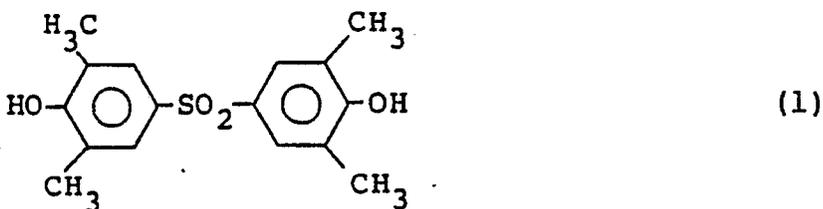
The compound acts as a charge control agent in the toner and is good in compatibility with a binder and the toners prepared using it are excellent in specific chargeability and good in charge durability due to moisture resistance.
