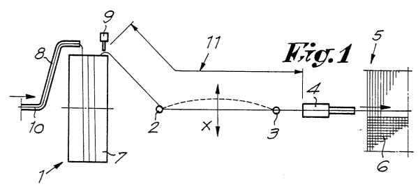
Method for adjusting the length of the weft thread to be inserted into the shed of weaving looms and devices used for this object.
