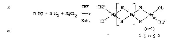
It is of course possible to prepare the THF solutions of Type I only at the cost of low hydrogenation 30 temperatures (0 °C), long hydrogenation times (18-20 hours), and incomplete conversion, which is a considerable drawback on an industrial scale.
